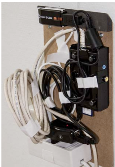
Figure 5. Raspberry Pi and Wi-Fi dongle (plus cabling) mounted in white boxes below the DIPs.
